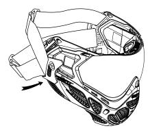
Insert the lens attachment buckles into the ear-holes on the side of the goggle system. (See fig. 3)
