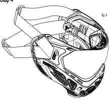
Place the anchor clip into the lens attachment buckle. The curved side of the anchor clip should be toward the rear of the goggle system. (See fig. 4)
