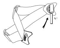
Connect headbands to lens attachment buckles by inserting the headband loop through the slotted opening on the buckle, and securing with the post. (See fig. 1)
