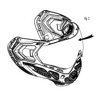
Insert the lens into the goggle system ensuring that the lens tabs are securely in place. The lens should be tight against the face of the goggle system. (See fig. 2)
