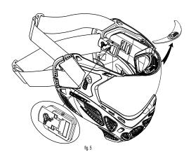
Lock the anchor clip into place by pushing the lever down toward the rear of the goggle system. Rotate dial into "LOCK" position. (See fig. 5)
